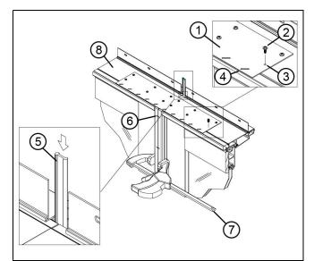
Figure 9 Inswing to Inswing mulling at head jamb
