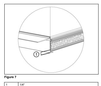
2. Position units together in desired mulling configuration. Check to be sure that frames at both sides of mullion are flush and nailing fin/drip cap kerfs are aligned. Lightly clamp units together on interior (use wood scraps to protect interior) near each end to hold
