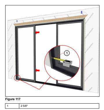
**7.** Snap the lower stationary bracket onto sill, then slide underneath the stationary panel until fully seated. The bracket should stick out approximately 2  $\frac{1}{4}$ " (57) from panel when fully seated. Fasten with #8 x 1/2" screw.See Figure 118.
