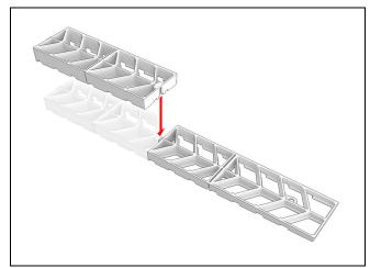
Figure 11 Connect counter-shims
