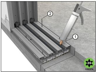
Figure 58 Seal and fasten HP sill.
