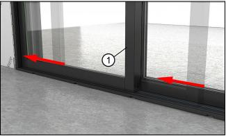
Figure 80 Move stationary panel tight against the jamb
