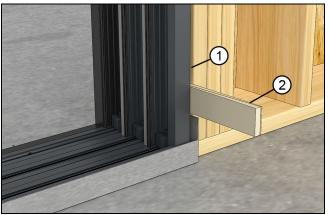
Figure 55 Center the frame and shim at stationary sill side
