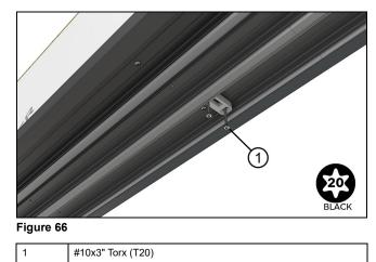
**6.** Install the remaining screws into the sill. (not provided on performance or flush sills). Fasten HP sills at 10" (254) on center. All other sills, fasten at 20" (508). See Figure 67. See Figure 54 previously for screw placement.
