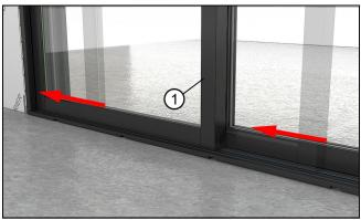
Figure 79 Move stationary panel tight against the jamb
