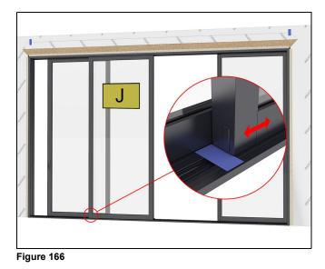
**9.** Close and lock the operator panel. The interlocks should engage and the stationary panel may move slightly. If the stationary panel did not move, firmly slide the stationary panel opposite the closing direction of the operator panel to fully engage the interlocks. See Figure 167.
