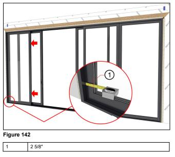
**13.** Snap the lower stationary bracket onto sill, then slide underneath the (C-L) stationary panel until fully seated. The bracket should stick out approximately 2 ¼" (57) from panel when fully seated. Do not fasten the bracket until all the panels are installed and adjusted. See Figure 143.
