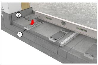
Figure 14 Level counter-shims with stackable shims
