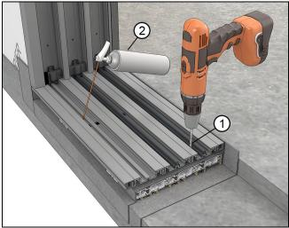
Figure 57 Drilling through HP stacked sill.
