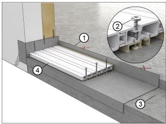
Figure 9 Install sill slope
