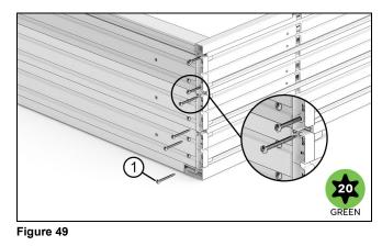
1 #8x1 3/4" self drilling screws (T20 Torx)
