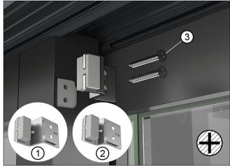
Figure 87 Top secondary panel bumper
