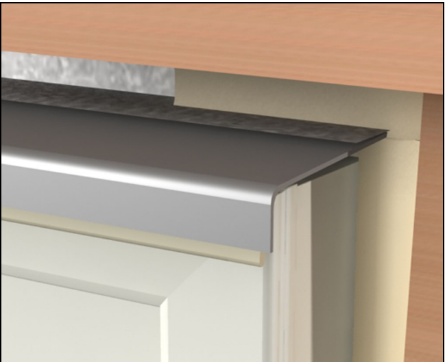
Figure 61 Apply sealant between unit and exterior finish at head jamb.
