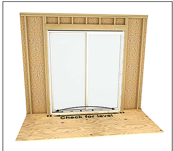
Figure 4 Start with a clean flat sill
