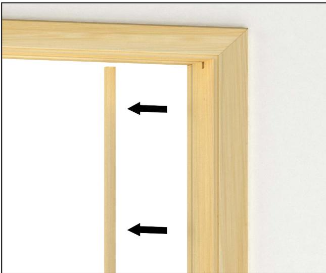
**Figure 6** Remove parting stops from side jambs
