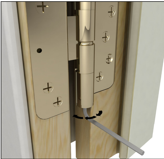
Figure 33 Lower the panel, counter-clockwise adjustment
