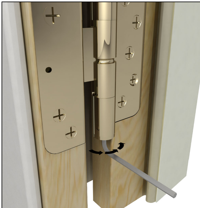
Figure 32 Raise the panel, clockwise adjustment
