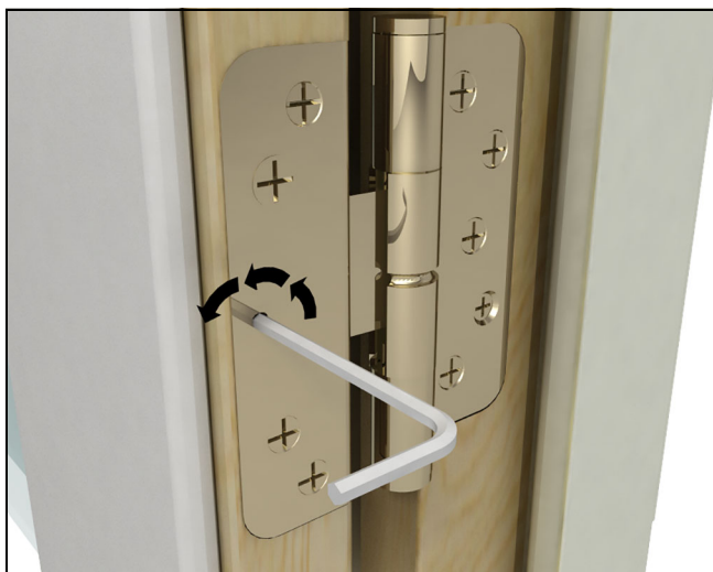
Figure 30 Counterclockwise to move panel away from jamb.
