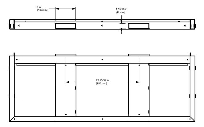
For ease of installation, all Skycove units come with the fork pocket dimensions shown above, regardless of call number size. These pockets can be used for equipment to safely lift the unit into the opening so it can be secured to the wall before the equipment backs away.
