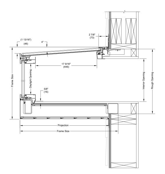
NOTE: Reference the Verification Document for specific Rough Opening reinforcement Typical wood frame construction shown. Refer to verification document for structural requirements. Measurement between bottom of cover to unit base.
