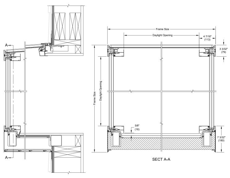
NOTE: Dimensions at glass. Due to projection and angle of side panels, the dimensions at the wall would Frame Size + X Tripane Glass only available on CN7870 units.
