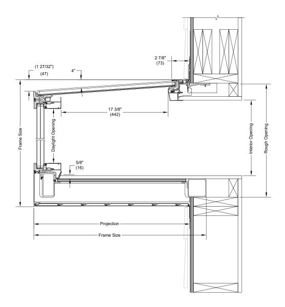
NOTE: Tripane glass only available on CN7870 units. Typical wood frame construction shown. Refer to verification document for structural requirements.
