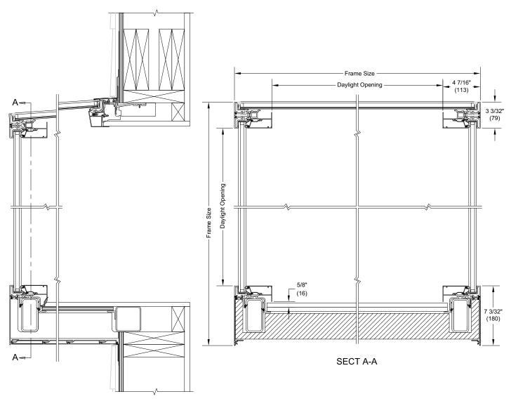
NOTE: Dimensions at glass. Due to projection and angle of side panels, the dimensions at the wall would Frame Size + X Typical wood frame construction shown. Refer to verification document for structural requirements.
