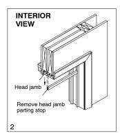
Remove the part stops from both side jambs and remove the top sash from frame. See illustration 3.
