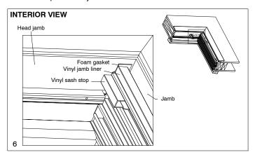
13. Install the wood jamb liner or sash stops that were removed earlier, using finishing nails. (Note: 1/4"(6) round moulding may be used in place of the wood jamb liner). Wood jamb liner and 1/4"(6) round moulding not provided.
