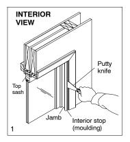
Slide the top sash down to the sill and remove the part stop from the head jamb. See illustration 2.
