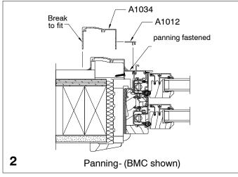
3. Break lines are provided on the panning components and may be used as a guide for cutting on a table saw or brake. See figure 3.
