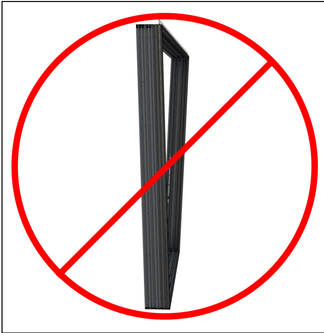
Figure 66 Make sure the entire frame is on the same plane and not twisted.
