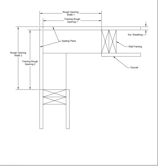
Figure 2 Framing Detail
