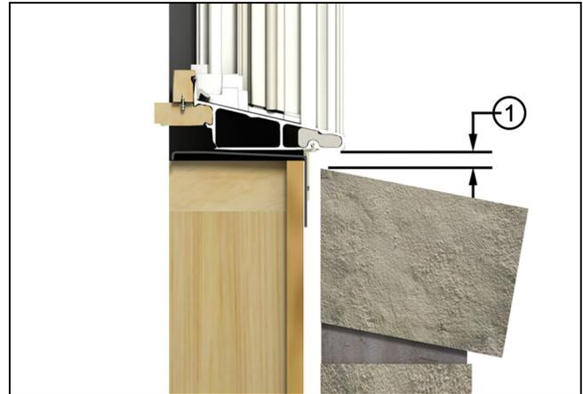
Figure 4 Avoid brick bind, maintain 1/2" gap
