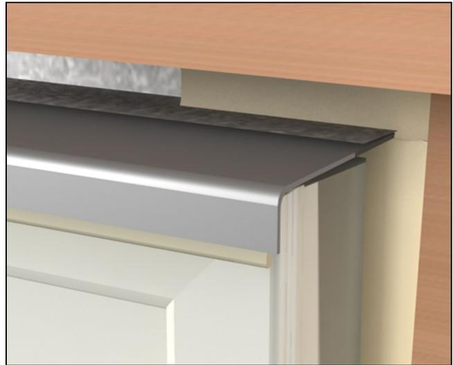
Figure 45 Apply sealant between window and exterior finish.
