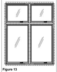
kerf. Make sure mulling pin is recessed at 1/4" on each end to allow for sealant application later. Insert remaining mull reinforcement boards between upper and lower assemblies. Fasten interior wood frame members with 1/2" x 1/2" 16 gauge staples spaced every 4" (102). See figure 13.
