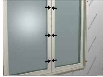
Figure 10: Adjusting the reveal between the sash
