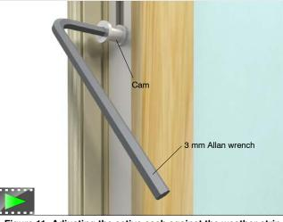
Figure 11: Adjusting the active sash against the weather strip
