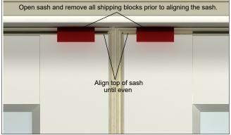
Figure 2 Adjust the top edges of the sash.
