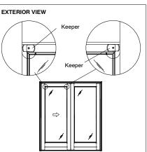
**IMPORTANT:** In the case of field applied exterior casing, it is imperative a 3/16" (5) reveal be maintained around the perimeter of the casing as shown in order for the combination assembly to fit properly. Please measure prior to installing combination panels. See illustration 2.
