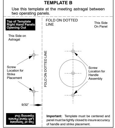
Combination for Ultimate Wood Inswing French Doors Installation and Finishing Instructions
