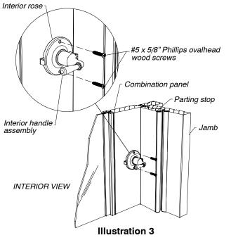
Predrill center bore with a 15/16" bit or hole saw and mounting screw pilot holes at handle locations using a 5/64" bit. Pre-drill pilot holes at strike locations using a 1/8" bit. Install interior handle assembly using #5x5/8" Phillips oval head wood screws. Do not over tighten. See illustrations 3.
