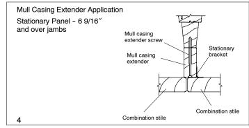
4. Place stationary panel into frame hold in place. Stationary panel brackets are to be installed 6" (152) from head jamb and sill and one at center on each stile. Hold the short side of the bracket against the combination panel and mark the holes on the stile. See illustration 5. Repeat at each location, remove combination panel. Apply stationary brackets to panel(s) using #7 x 3/4" Phillips head screws as shown in illustration 5.
