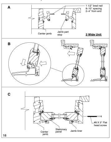
Attach the wood panel guide (with its applied tape) to the three wide non-interlocking panel. Fasten with 1 1/2" (37) finishing nails every 8" (203).
