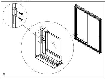
16. Use a stiff putty knife to bend the head jamb bracket into place. See illustration 10. Fasten the head jamb bracket to the head jamb with two "H" #8x1" flat head screws placed at a 45° angle. See illustration 10.
