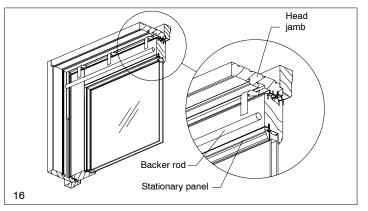
Insert stationary cover dust block end over interlock and slide into place. Fasten the stationary cover(s) into the head jamb with three #8X1 1/2" flat head screws "C" into the predrilled holes. See illustration 17.
