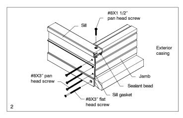
5. Using the predrilled holes in the sill, drill through the sill and into the side jamb approximately 3" (76) with a 3/32" drill bit. Beginning with the hole closest to the sill liner, fasten the sill to the side jamb with #8 X 3" Phillips pan head screws "E". Fasten the sill to the jamb casing with #8 X 3" Phillips flat head screw "B".
