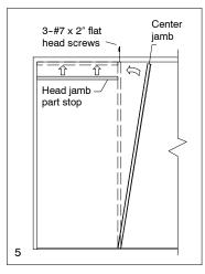
With help, stand frame up to vertical position. For ease of assembly temporarily install unit into opening and fasten the top corner to the structure.
