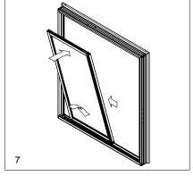
14. Push the bottom of the panel outward and gradually tilt panel to the upright position. Press the panel outward ensuring that the flange on the panel leveling block has fully seated into the sill clip and slide panel to the vertical jamb. See illustration 8.
