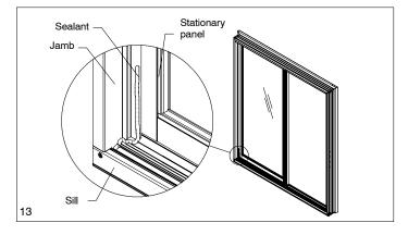
Attach wood interior stationary jamb cover(s). Install wood interior jamb liner, bevel side towards panel. See illustration 14.
