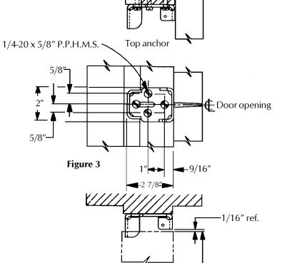
Cut off top end of mullion body so length is 1/16" less than this dimension
