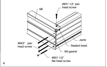
Apply a bead of sealant from the bottom of the sill along the jamb up 8- 10", sealant must adhere to the Ultrex, wood and cladding joint. See illustration 5a. Cover sealant with 2" masking tape to avoid contamination. See illustration 5b.
