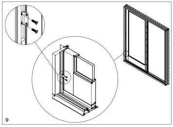
16. Use a stiff putty knife to bend the head jamb bracket into place. See illustration 9. Fasten the head jamb bracket to the head jamb with two "H" #8x1" flat head screws placed at a 45° angle. See illustration 10. For two wide units proceed to step 20.
