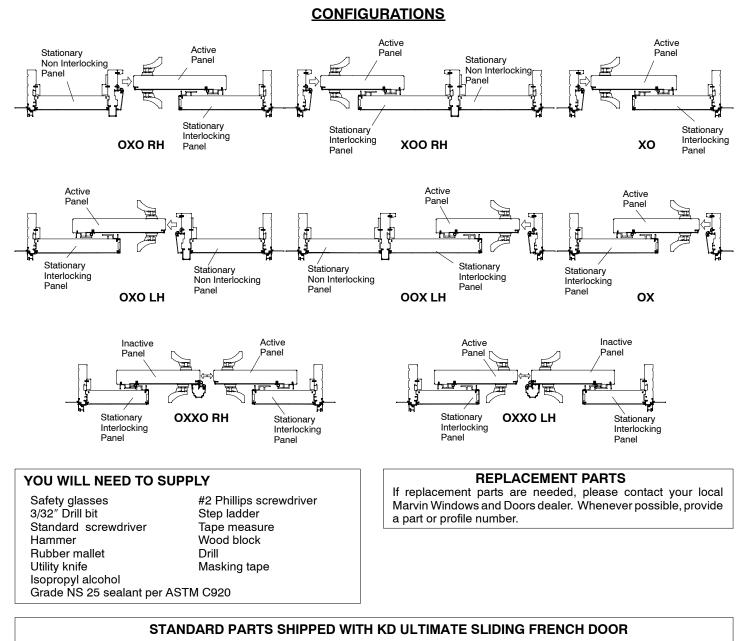
2- wide assemblies include: 1- head jamb, 1- sill, 2- side jambs, 1 - active panel, 1 - interlocking stationary panel.
