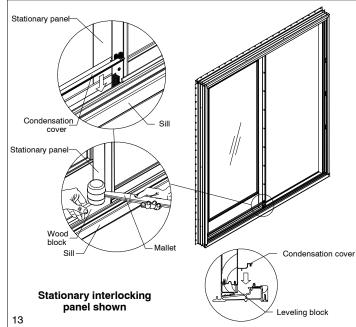
20. Apply a 3/16" to 1/4" bead of sealant over the condensation cover and up the jamb 8- 10". See illustration 14. Also apply sealant on the non interlocking side of the center jamb for OXO units. Apply to both sides of the center jamb if XOO or OOX configurations.
