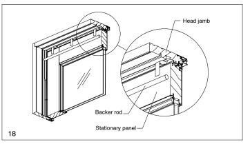
24. Insert dust block end of stationary corner over interlock and slide into place. Fasten the stationary cover into the head jamb with #8X1 1/2" screws into the predrilled holes. See illustration 19.
