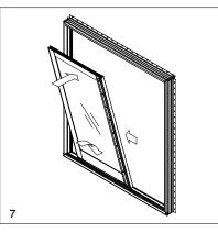
14. Push the bottom of the panel outward and gradually tilt panel to the upright position. Press the panel outward ensuring that the flange on the panel leveling block has fully seated into the sill clip and slide panel to the side jamb. See illustration 8.
