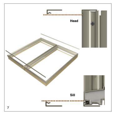
11. Run a 1/4" (6) bead of sealant/adhesive on top of mull blocking at edge of mull and sides approximately 2 1/2" (64) back. Cut appropriate width pieces of foam block and press into adhesive as shown in illustration 7 to both ends of the mull.
