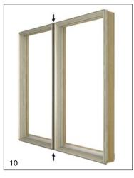
14. Place mull cover even with interior edge of frame trim as shown and carefully tap onto frame with a plastic headed hammer and wood block. See illustration 11. Proceed to step 18.
