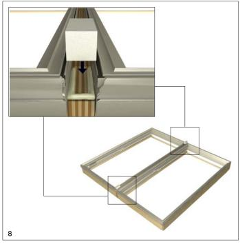
12. Lay another bead of sealant on top of foam block even with cladding as shown in illustration 9.
