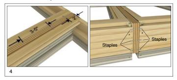
6. Turn the unit over and apply the exterior mull casing per the following exterior space mull instructions for Clad Units; for Wood units proceed to step 14.
