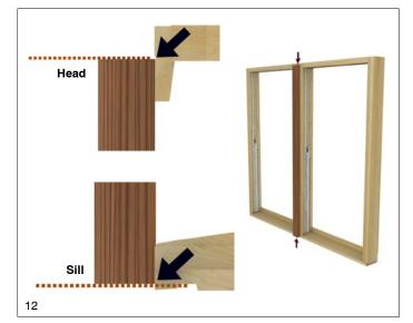
16. Measure width of the unit plus width of exterior casing and cut and notch subsill to length. Treat any cut parts with a water repellent wood preservative. Apply sealant next to the kerf on the subsill and secure subsill to sill with #8-15 x 1 3/4" wood screws placed per illustration 13.
