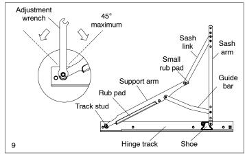
NOTE: Do not rotate track stud more than 45 °from perpendicular in either direction.
