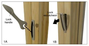
NOTE: When re-installing the lock escutcheon, be sure the top of the escutcheon is applied first and then push on the face of the lock escutcheon from top to bottom with one motion until a firm "click" is heard. Push the lock handle onto the lock base until a firm "click" is heard. See illustration 1C.
