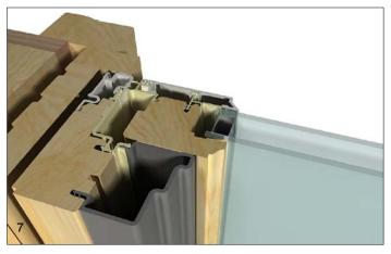
2. Repeat for the other stop and install the head jamb and sill stops.
