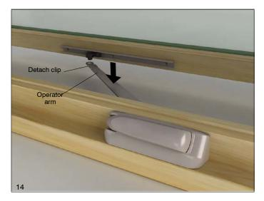
CAUTION: To avoid damage to the sash and/or personal injury, the awning sash must be fully supported at all times. Do not lift sash past 60 degrees with the hinge arms attached. Do not rack the hinges during removal, the sash rail must remain parallel to the head jamb when removing or installing the sash. Do not tip or rest the sash on the corners.
