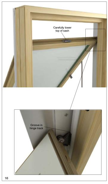
5. To reinstall the sash reverse the sash removal procedures. Keep the sash shoes flat up against the track just in front of the groove. Keep the sash stile parallel to the sill slide the sash shoes into the groove in the track. The sash should be fully supported until both shoes are securly engaged with the hinge track and the hinge arms are placed onto the hinge stud and clips seated. See figures 15 and 16.
