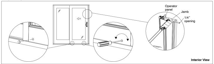
Figure 2: Adjusting the panel.
