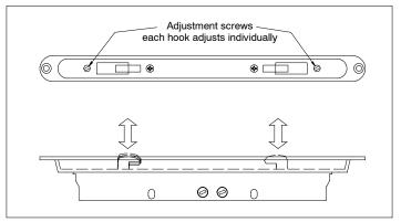
Figure 4: Adjusting hooks.
