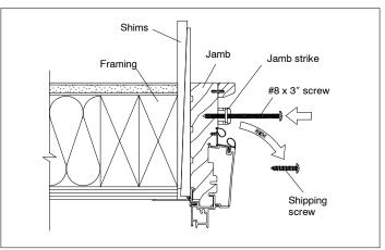
Figure 3: Installing screws.
