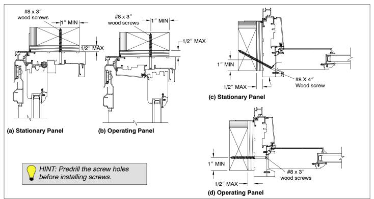
Figure 1: Securing the door.
