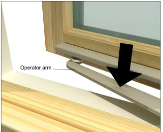
Figure 1 Detach operator arm.
