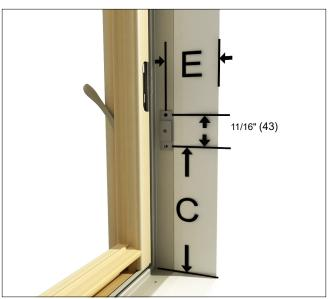
**Figure 9** Clad frame (also applies to wood frame). Applies to Casement jamb.
