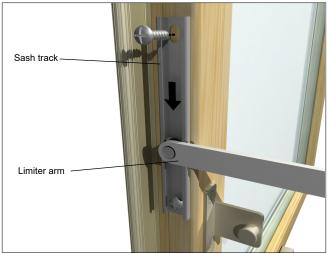
Figure 11 Install the sash track and limiter arm.
