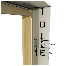
Figure 10 Clad frame shown (also applies to wood frame). Applies to Casement jamb and Awning sill.
