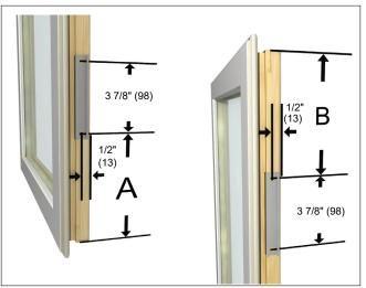
Figure 8 Casement sash shown. Applies to Casement stile (A and B) and Awning bottom rail (B).
