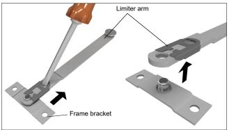
Figure 7 Disconnect and remove frame bracket.
