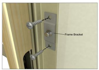
Figure 12 Fasten the frame bracket to the frame.
