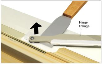
Figure 2 Detach hinge linkages.
