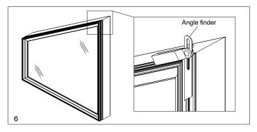
9. Place CBMC on with inside frame corner of mitered end on outside corner of unit frame. Temporarily place next CBMC (that will join with previously cut CBMC) so that it touches the inside corner as shown in illustration 7.
