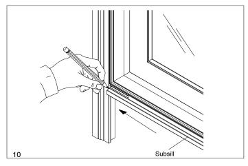
14. Use a straightedge and mark the bottom of the casing as shown in illustration 11 ensuring the subsill is pushed firmly against the sill.
