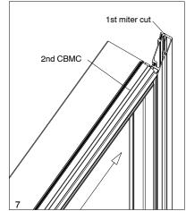
Using a straightedge, transfer the angle to the second CBMC 10. as shown in illustration 8. Remove and cut the angle scribed on the CBMC with a power miter saw. Ensure the cutting line remains visible.
