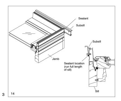
For door products, apply silicone sealant from the top edge of the jamb cladding at the sill to beyond the jamb accessory kerf as shown in illustration 15.
