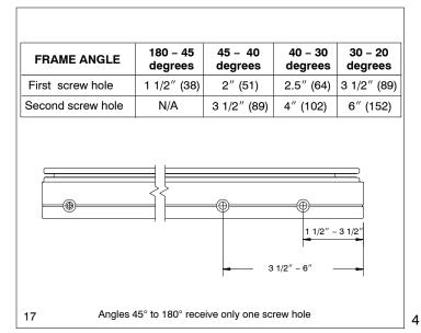
21. Fasten corner key to CBMC using a #8 x 5/8" flathead screw to first hole and if necessary a #8 x 1 1/2" flat head screw to second hole. See illustration 18.
