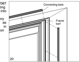
24. Install CBMC assembly on frame. Press CBMC into connecting barb and kerf by hand then secure firmly with a rubber mallet. See Illustration 21.
