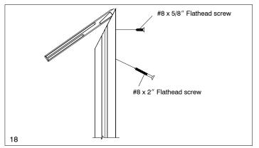
22. Assemble all CBMC components in the same manner as described in steps 18–20. Make sure all miter joints are tight. See illustration 19 –21.
