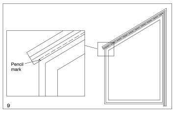
Once all sides have been cut to fit properly, remove all CBMC except those pieces which will extend down to the sill. Temporarily install subsill (window products only) and slide against the inside of the CBMC as shown in illustration 10.
