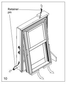
11. To install the insert unit from the exterior, place the insert unit into frame, head jamb first. Then, swing the sill end into place. Secure unit by putting in the two frame retainer pins. See illustration 11.
