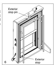
Remove the two frame retainer pins and carefully pull the bottom of the insert out to the exterior to remove unit from frame. See illustration 7.
