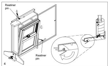
Pull out on the spring loaded interior stop pin and swing the interior stop into place and release the pin. See illustration 5.
