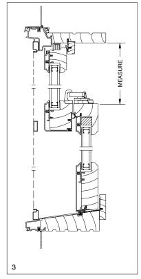
NOTE: Two lineal length stationary filler blocks are sent with notches on both ends. When cutting blocks, only one notched end is needed per jamb. However, these blocks must be handed (notches must fit around the head jamb parting stop). Cut blocks individually to fit around head jamb parting stop.
