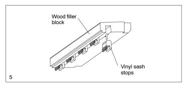
Snap filler blocks into jamb carriers. The connecting barb on the vinyl sash stops will fit between the jamb stop and the top sash balance tube. Take care not to damage bottom sash check rail and head jamb. See illustration 6.
