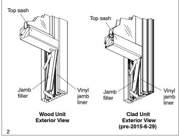
NOTE: On wood units with ogee lugs jambs filler will have to be cut to fit around lug.
