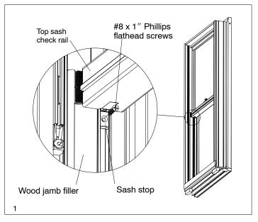
Snap the jamb carrier fillers into the exterior balance tube cavity as shown in illustration 2. For ease of installation, insert top of filler first and snap into place. Be careful not to mar the sill or top sash checkrail. Replace bottom sash (see installation instructions).
