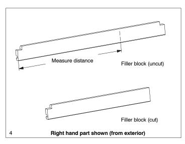
4. When the filler block fits properly, remove from unit and insert the vinyl sash stops at even intervals into the channel on the back of the filler blocks as shown in illustration 5.
