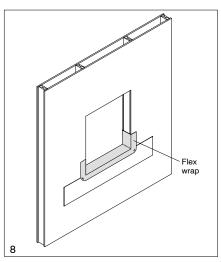
NOTE ON PANNING THE SILL: If a flexible adhesive membrane is not used to pan the sill, be sure to properly seal the bottom corners of the rough opening. Then use regular adhesive membrane along with relief cuts to properly pan the sill. If pan flashing is to be used, install now.
