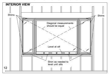
14. When window frame is square and plumb, nail through the jamb nailing fin a maximum of 6" from the upper corners. Do NOT drive nails all the way in. See illustration 13. If your unit is secured by brackets\* start at the interior upper corners and attach with two #8 x 1 1/2" flathead wood screws.
