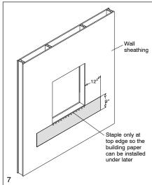
Use appropriate width flexible self sealing adhesive membrane to pan the sill. Make the piece long enough to ride up the jambs at least 4" (102) on each side. Fold the wrap out onto the exterior as shown in illustration 8. Staple exterior corners of the sill panning to hold the wrap in place until the adhesive cures.
