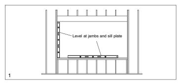
When framing rough opening, obtain dimensions from unit as shown in illustration 2. Masonry openings (MO) should be 1/2" (13) wider and 1/4" (6) higher than outside measurement of frame.
