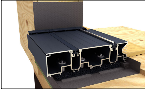
Open face slot with wood construction. Slot recess is 3/8" (10). Available flooring is 2" (51) however 3/4" (19) hardwood flooring is used leaving 1 1/4" (32) sill face exposed.
