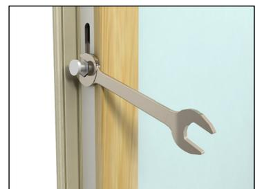
Figure 5 Adjusting the cam.
