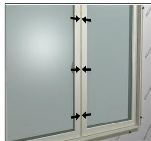
**NOTE:** Top and bottom sash hinge movement is independent. Adjust each hinge accordingly.
