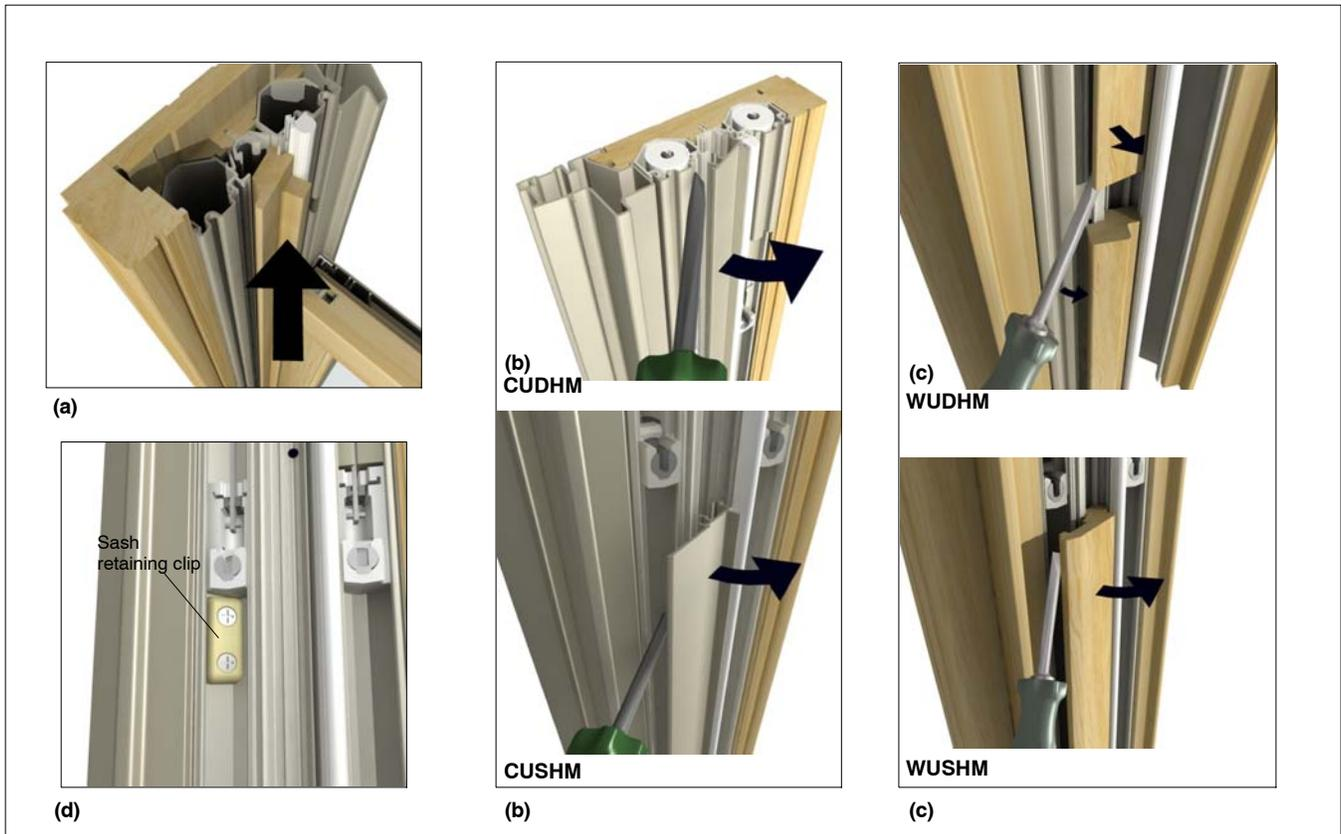
Figure 3: Removing Jamb Fillers
