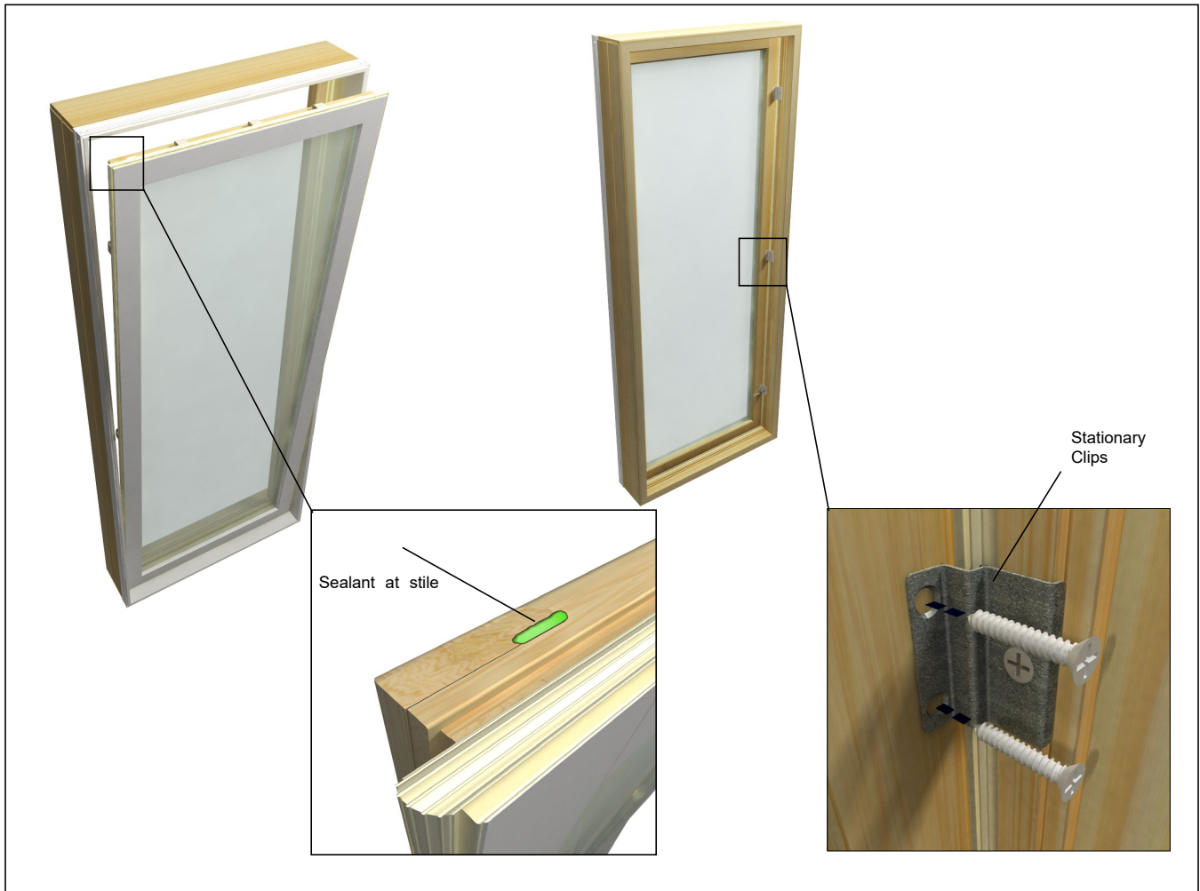
Figure 3 Installing stationary sash and fastening in frame.
