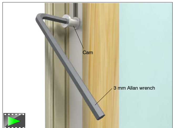
Figure 11: Adjusting the active sash against the weather strip
