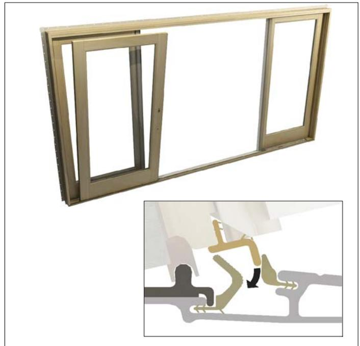
Figure 7: Units with low profile sill.
