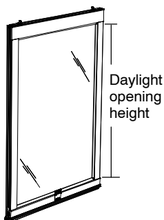
Top Sash Interior View
