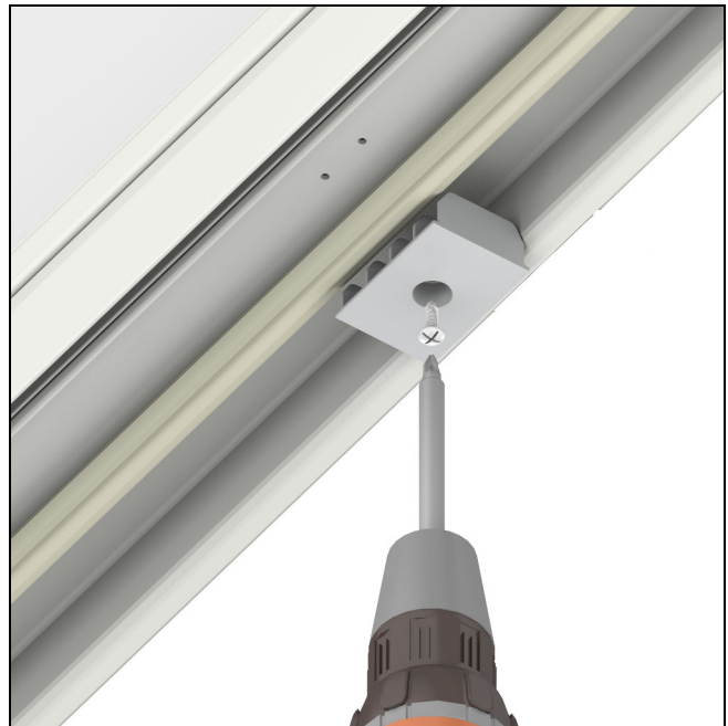
Figure 5 Secure blocks through head jambs with 5/8" screws.
