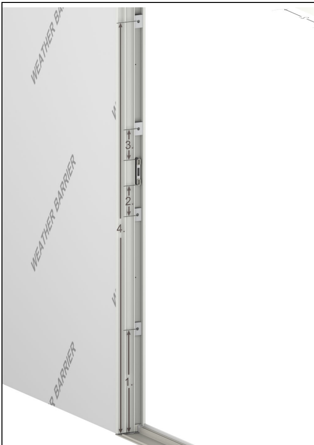
Figure 3 Block Placement for Operator Jambs.
