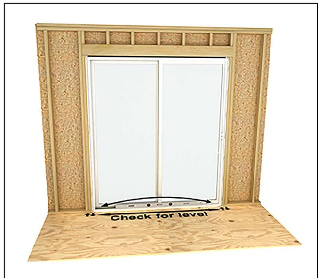
Figure 3 Start with a clean flat sill
