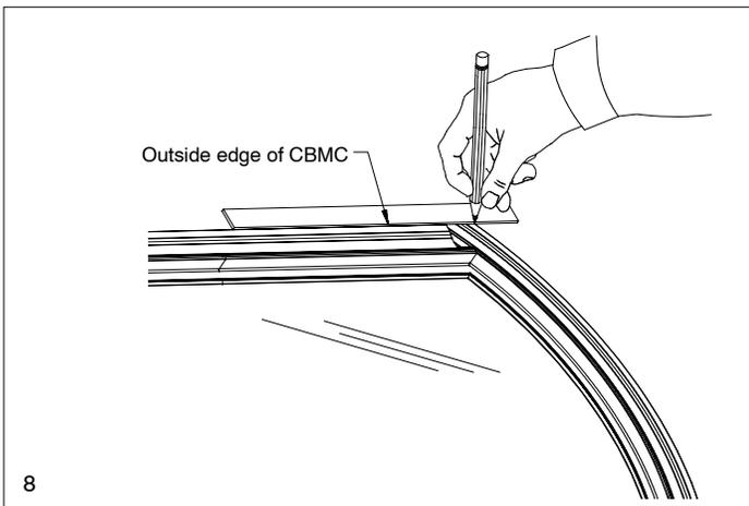
11. For applications that require a spliced joint mark parallel with mull cap, approximately 3/8" (10) below the mull cap. See illustration 9. For spring line applications measure 1" (25) from the spring line (where the radius stops) on the exterior of the radius CBMC on both sides and mark in a parallel fashion.
