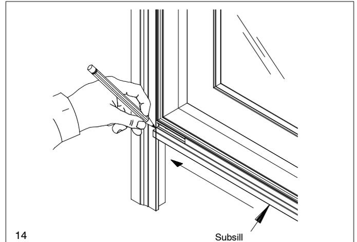
17. Use a straightedge and mark the bottom of the casing as shown in illustration 15 ensuring the subsill is pushed firmly against the sill.
