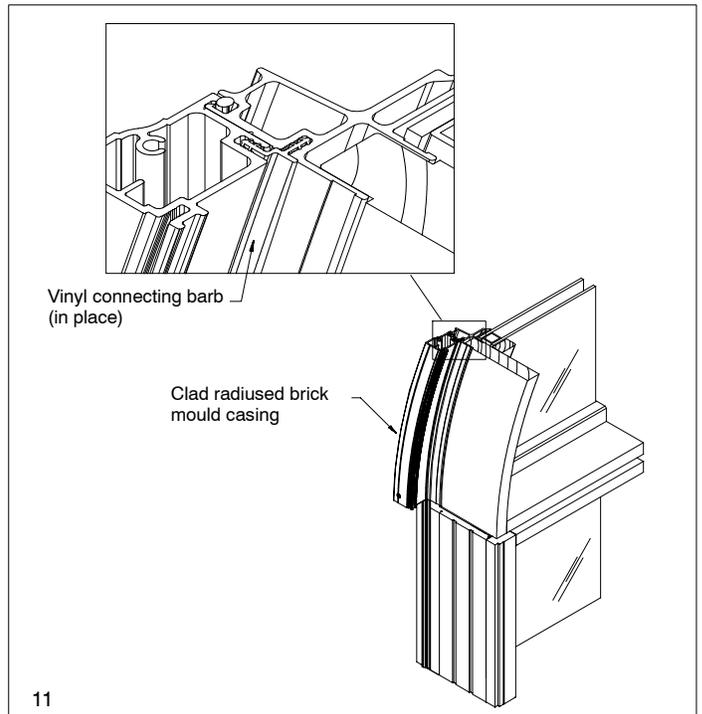
14. Temporarily install jamb CBMC making certain that the top of jamb CBMC touches the radius portion as shown in illustration 12.
