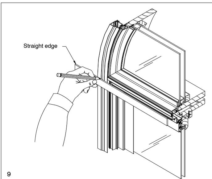
12. Using a straightedge, intersect the two lines to mark the angle needed to be cut as shown in illustration 10. Remove radius CBMC from frame. Place a 1" x 3" x 3/16" shim under the CBMC to provide support while positioned in the power miter box as shown in illustration 10. Cut the angle making sure the cutting line remains visible.
