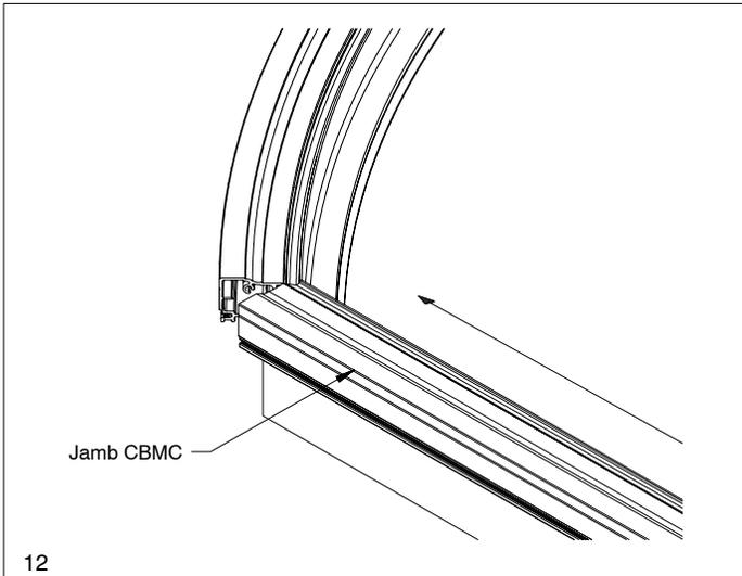
15. Using a straightedge, transfer the angle on the radius portion to the jamb CBMC as shown in illustration 13. Repeat this procedure for both jamb CBMCs. Remove and cut the angle scribed on the CBMC with the power miter box saw. Ensure the cutting line remains visible.
