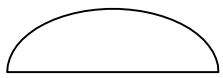
Half Ellipse Made using two or more radii. Also called compound radii ellipse. Not true radius.
