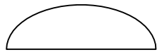
Made using two or more radii. Also called compound radii ellipse. Not true radius.
