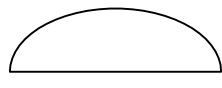
Half Ellipse Made using two or more radii. Also called compound radii ellipse. Not true radius.
